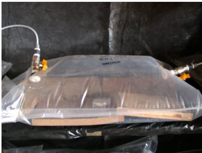
Figure 1. Closed plastic container (Gas Bubble) with non-toxic physical controls such as CO 2 , or N 2 gas.
