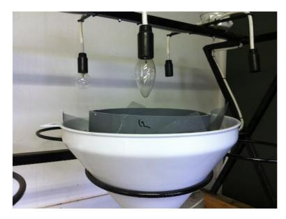
Four small spacers are used to elevate the sieve above the funnel to facilitate airflow. I use wooden clothes pegs (removing the metal spring and using the two bits of wood as two spacers:
