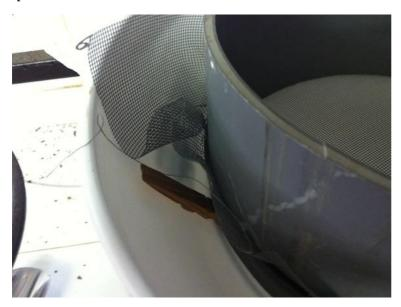
A 50ml falcon tube (or similar), approximately 1/3 full with ethanol, is pushed onto the end of the funnel:
